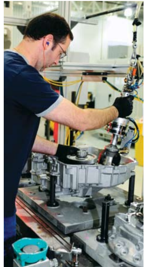
Tom Morisette assembles the new front-wheel-drive transmission at the Van Dyke Transmission Plant in Sterling Heights, Mich. Below, one of Ford's new fuel-efficient, 6-speed transmissions.
