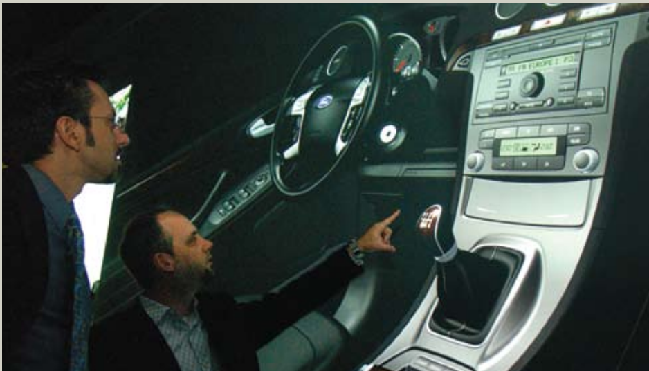
Virtual tools allow full-scale review and refinement of computerized vehicle designs.
