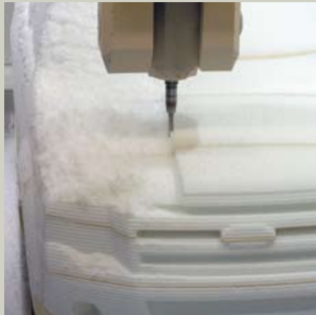
Modeling mill sculpts full-scale prototypes.
