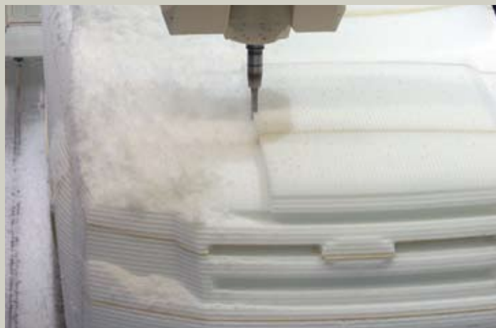
The milling machine allows Ford to do more model sculpting in less time.
