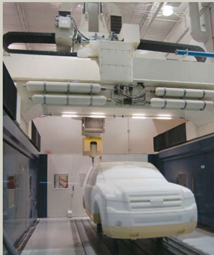
Ford’s new milling machine can create full size models of vehicles as large as the F-350 Super Duty pickup.
